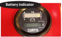
Battery indicator and hour indicator for hours remaining before next service.
