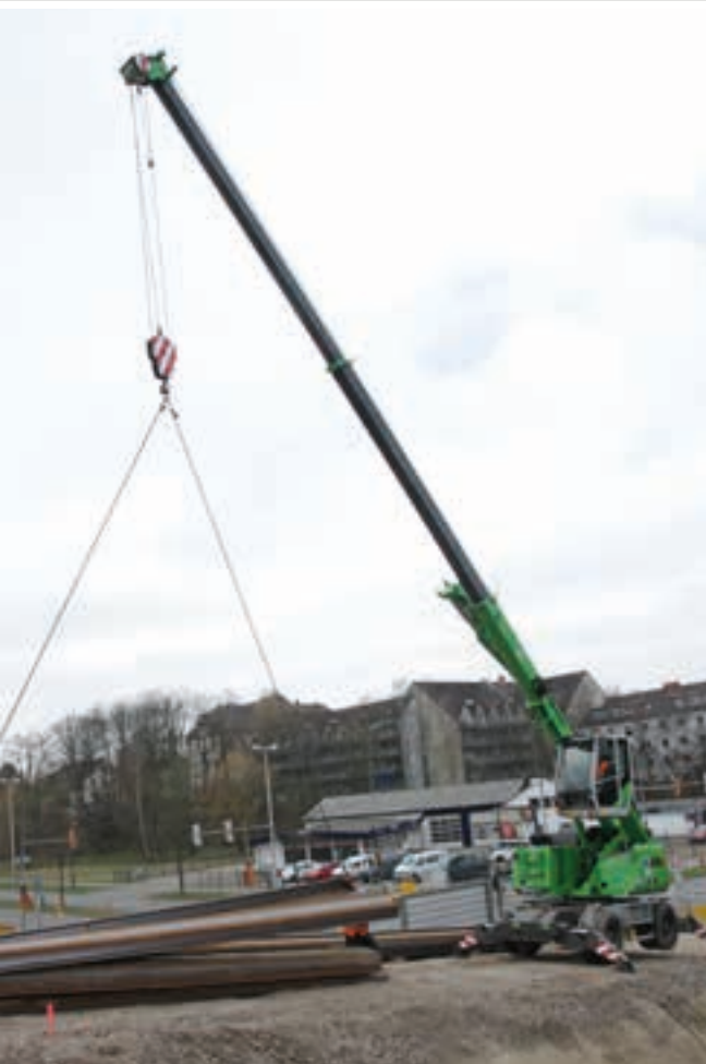
The 613 E Mobile being used for lifting activities and logistics tasks at a railway construction site
