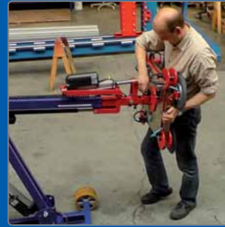
The vacuum suction arrangement is screwed for safety reasons.
