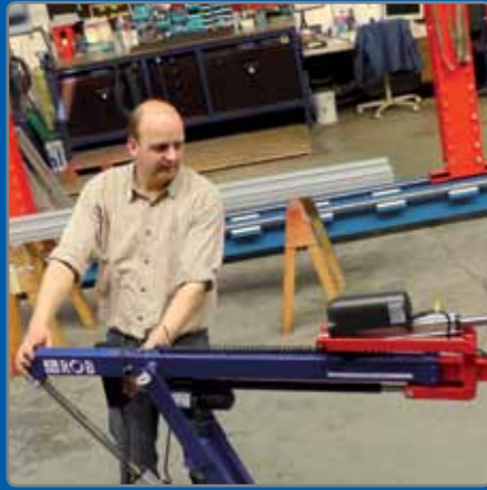
The telescope arm is pocketed and the cylinder connected.
