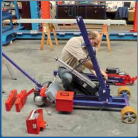
Chassis, axis and hoist mast become in the first step mounts.
