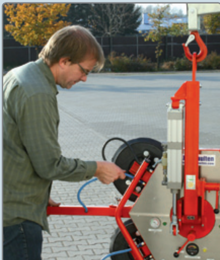
Easy reconstruction and widening of suction plates to get a higher load capacity.
